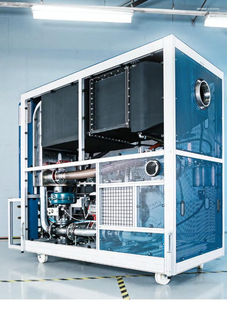
Moisture in natural gas can damage the sensitive equipment at natural gas fuelling stations, reduces efficiency and increases the emissions from combustion engines. In a joint project with RAG Rohöl-Aufsuchungs AG, Christof Systems has developed a natural gas dehydration facility.
